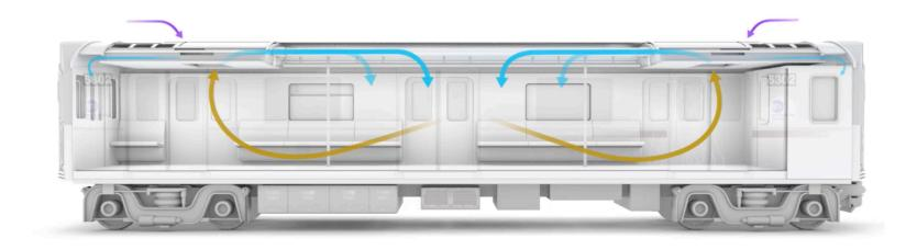
At the same time, outside air is pulled into the system, combined with the existing mix and released into the car through the duct panels, which span the ceiling.
